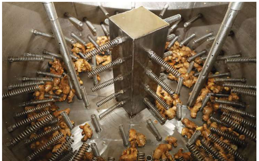
The Ginger washer at the Spice Processing Facility in Region 1
